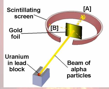
[A] Particles going through the foil [B] particles scattering
