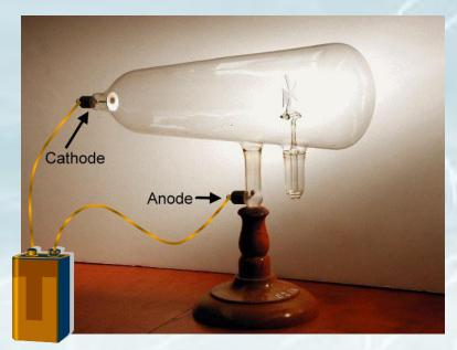
This shows that the source of light is the cathode. The light is called a cathode ray
